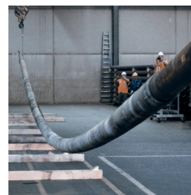
Polyurethane (PUR) field coating before and after bending
