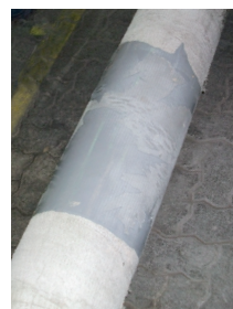
Polyurethane (PUR) field coating before and after bending
