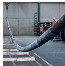
Polyurethane (PUR) field coating before and after bending
